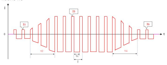
AC TIG welding current waveform
