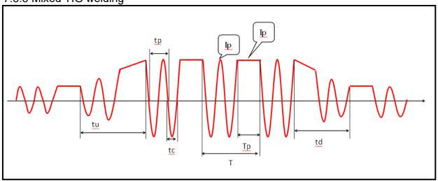
Current waveform of mixed TIG welding
