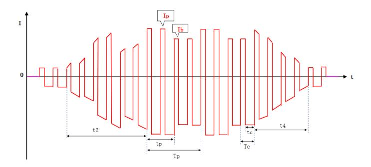
Current waveform of AC pulse TIG Welding
