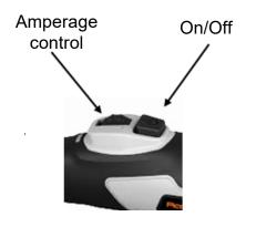
5. When using the Analog TIG welding torch, set the parameters on the panel to your desired Min and Max amperage range. During Welding the Amperage control dial can be used to adjust the welding current from the minimum to the maximum set value (Base/Peak amps)When you wish to stop the welding process press the on/off button or simply lift your Tungsten off the work to break the current continuity.
