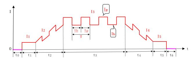
DC pulse TIG welding current waveform
