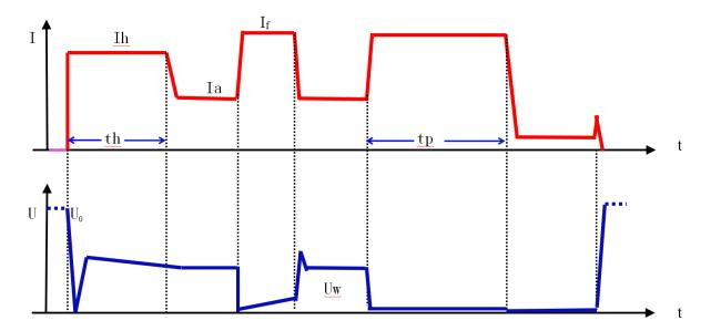
ARC electrode welding process
