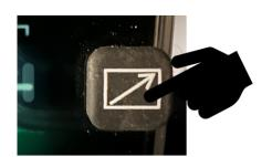
3. Under no load, press the key to turn the indicator on. At this time the remote Torch controller is in remote
